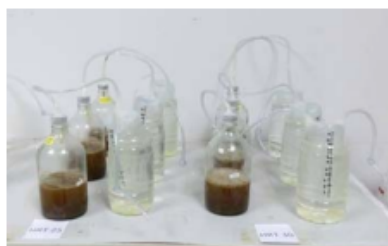
Fig. 1 Batch digestion experiment at different hydraulic retention time studied in this work.
