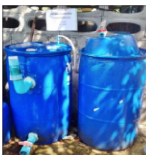
Fig. 2 Continuous digestion experiment at the pilot scale.
